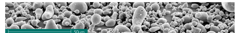
SEM aspect of SN2383 atomized tin powder
